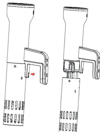
**NOTE!** never run the appliance without securely fastened the metal cover.
